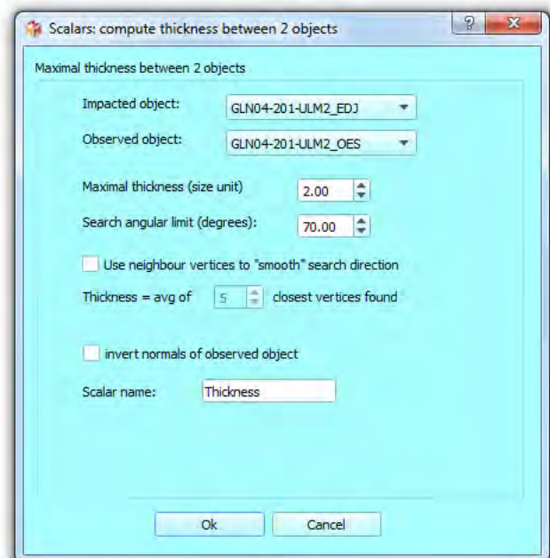
Figure 11.11: Thickness between 2 surfaces window
